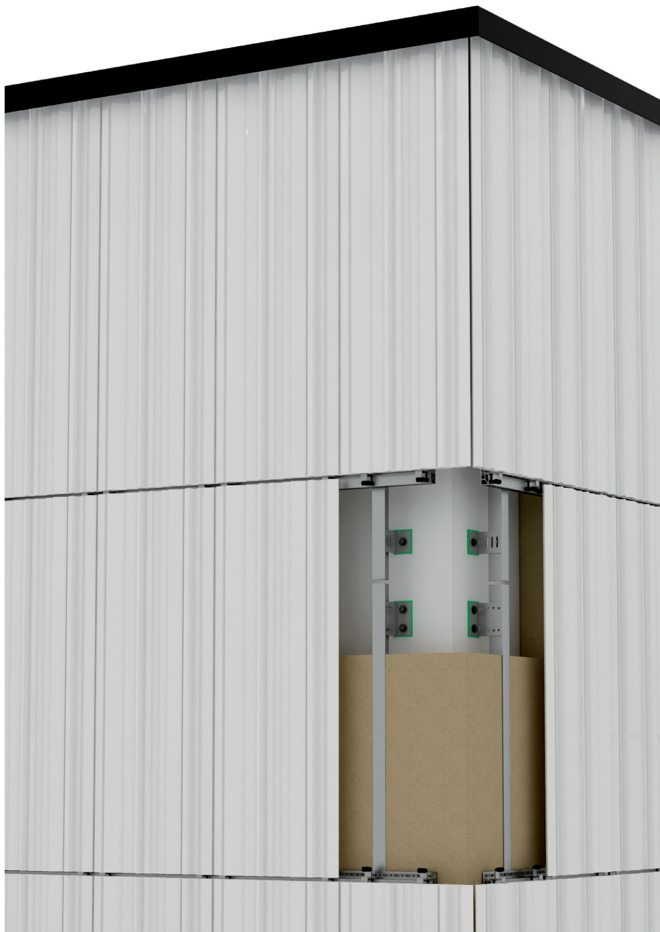
Corner detail • Detalle esquina
